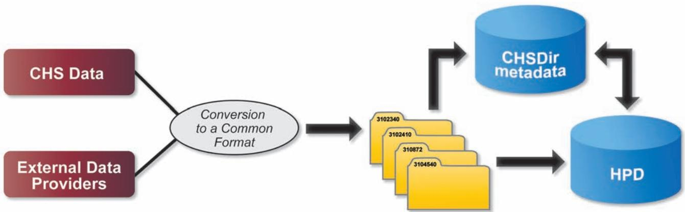
(Above) A simplified representation of the file-based workflow for the bathymetric data management.
